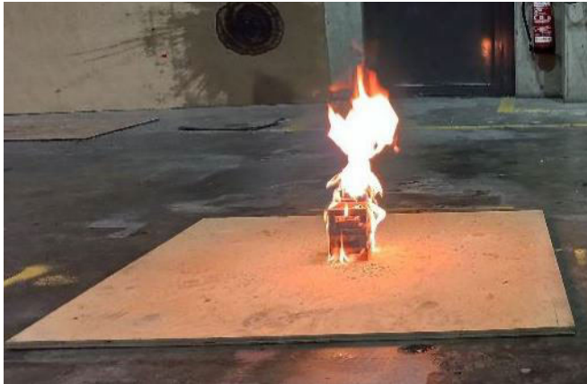
Figure 7: The wood crib screwed on a wooden board and set on fire
