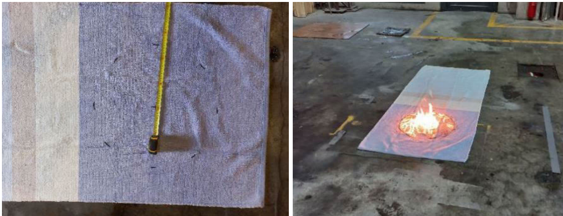
Figure 1: The outlined circle in which the kerosene was spread (left) and after the kerosene was set on fire (right) on the bath rug.
